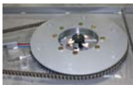
DuraGlide cams and a precision ring bearing reliably support 5,000 pound loads on the LPE.
