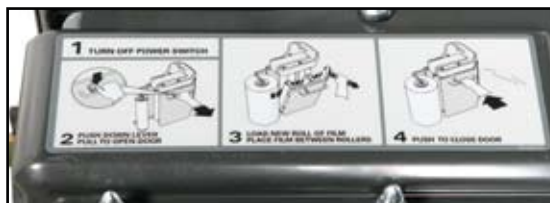
Graphic instructions on top of the carriage guide the operator through film threading.
